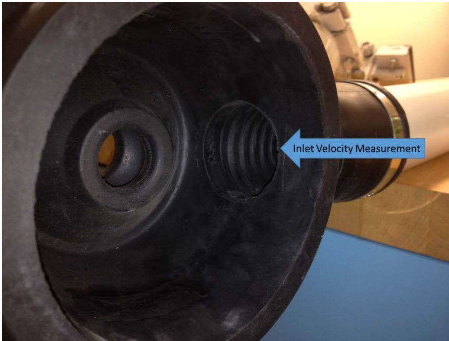
Figure 3.9 Inlet velocity measurement location on the DustControl® pneumatic rock drill hood
