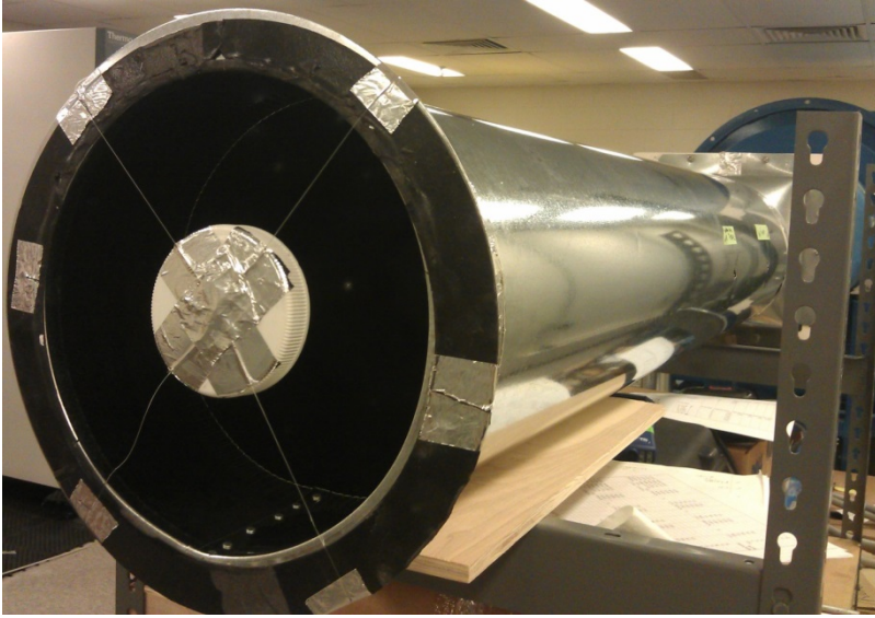
Figure 2.6 Flanged novel design 4 (ND4)
