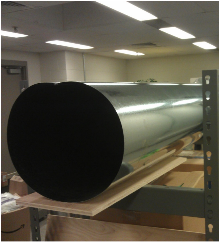
Figure 2.1 Unflanged traditional LEV inlet design (Traditional)
