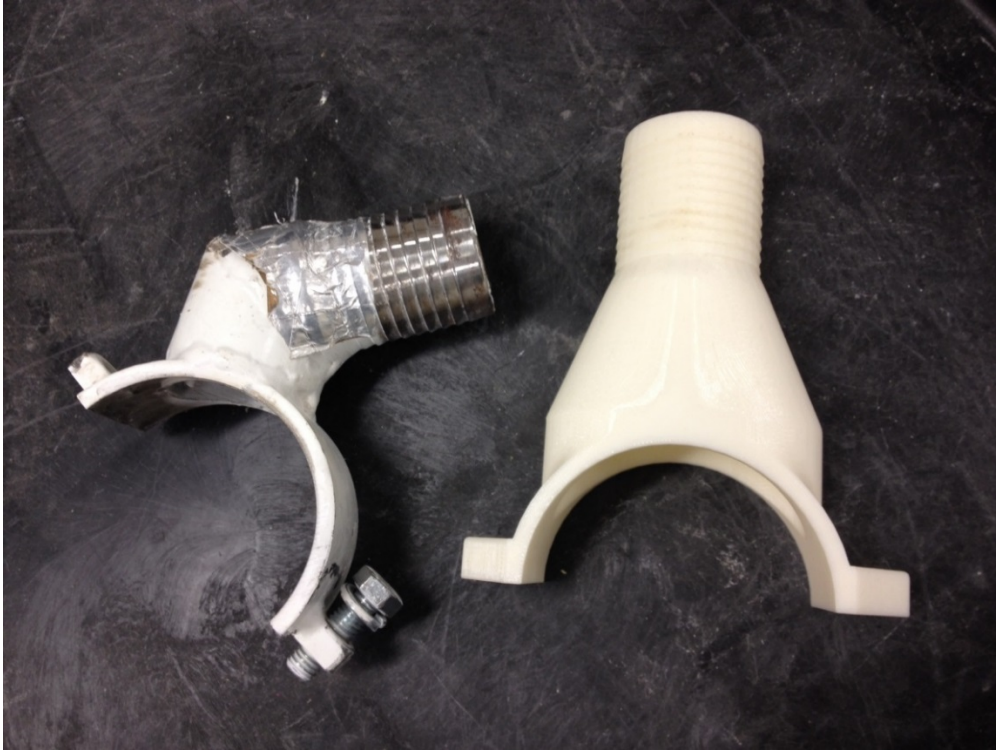
Figure 3.7 Minnich and NIOSH prototype simple hoods after removal from enclosing housing
