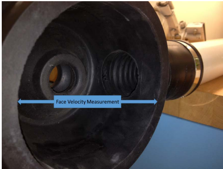
Figure 3.10 Face velocity measurement location on the DustControl® pneumatic rock drill hood
