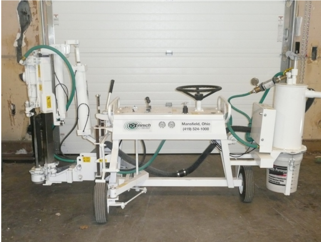
Figure 3.1 Minnich A-1C Single Drill, On Slab Unit with optional dust collection system
