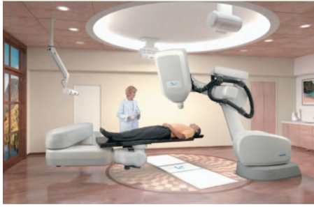
FIG. 1. CyberKnife image-guided radiosurgery system with robot-mounted linac, patient couch, dual orthogonal imaging detectors in the floor, and dual x-ray imaging sources mounted at the ceiling. (Image courtesy of Accuray, Inc.)
