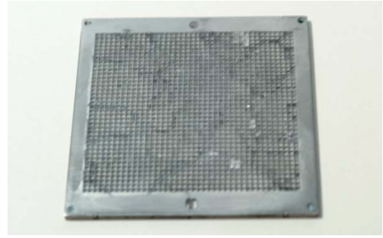
FIG. 2. Segmented detector prototype consisting of CsI(Tl) injected into a 2 mm thick tungsten matrix of 40 \times 40 cells of 1 mm pitch and a septal wall thickness of 50 \mu\text{m} (equal to that used in the theoretical calculations).
