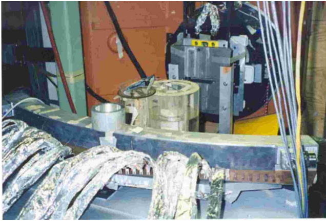
FIG. 21. Benchtop tomotherapy prototype system incorporating a NOMOS collimator (courtesy of T. Mackie).
