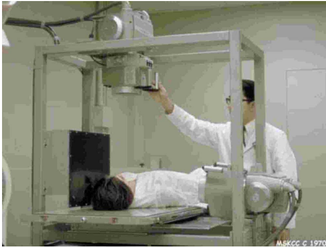
FIG. 17. Apparatus for the automatic localization of implanted seeds c 1970 (MSKCC).
