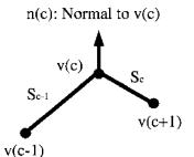
FIG. 3. The vertices of the polygon and positions used in the active contour model.
