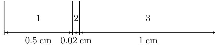
Figure 2.10: Graphic depicting geometry of analytic 1-D slab problem with material labels 1, 2, and 3 corresponding to materials with \Sigma_{t,1} = 1 , \Sigma_{t,2} = 100 , \Sigma_{t,3} = 0.5 , respectively.
