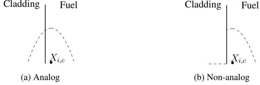
Figure 2.1: Graphic depicting analog (right) and non-analog (left) view of fission reaction rate estimation using KDEs. X_{i,c} indicates a fission or collision site with the dotted line representing the kernel associated with that event.
