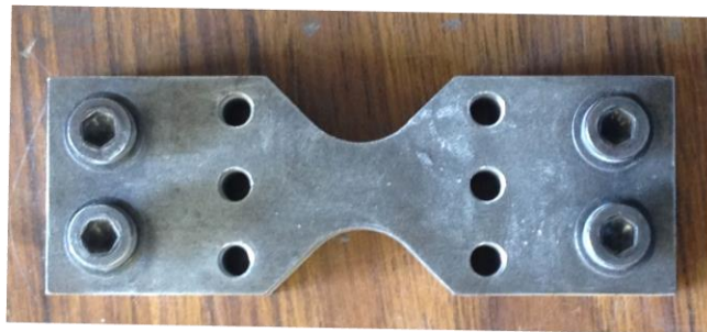
Figure 3-2. Template used for small Arcan specimen fabrication.
