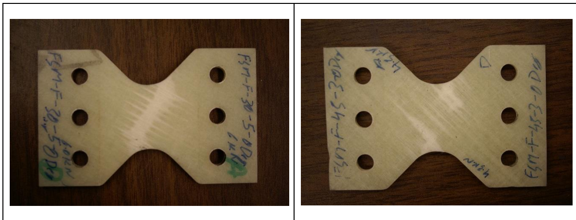
Figure 4-14: (Left to right) Failure surface of small 30° and 45° off axis specimen at 0° loading angle.
