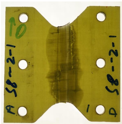
Figure 3-10: Failure surface of a 2-1 specimen subjected to shear load ( \alpha = 90^\circ ).
