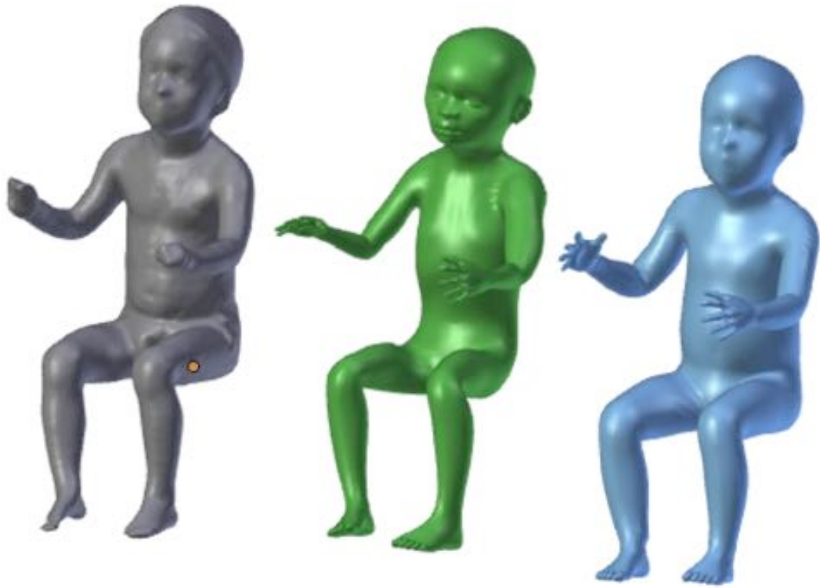
Figure 32. Scanned body shape (A). Template manikins originally generated from the MakeHuman software (B) and template generated using bootstrap technique (C).
