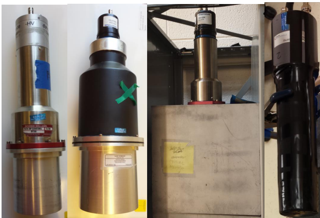
Fig. 2-7. Examples of the detectors used in measurements in this dissertation including from left to right: 7.62 cm \emptyset EJ309 organic liquid scintillation detector, 12.7 cm \emptyset EJ309 organic liquid scintillation detector, 25 cm by 25 cm by 10 cm BC501A organic liquid scintillation detector, 5.08 cm \emptyset stilbene crystal couple to PMT (5.08 cm \emptyset BB3 plastic scintillator looks identical when wrapped and coupled to PMT). Pictures are not to scale relative to each other.
