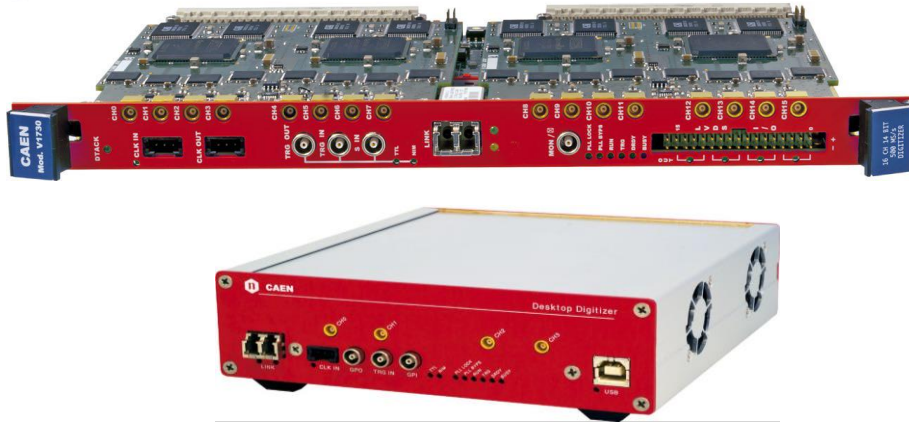
Fig. 2-9. CAEN V1730 (top) and DT5720 (bottom) digitizers.
