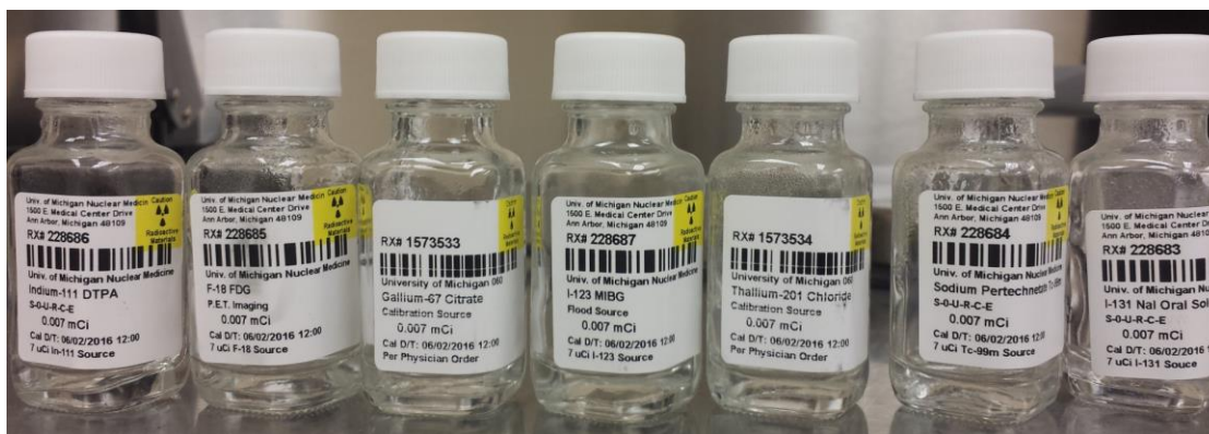
Figure 5-10. 7 – 8 \mu Ci medical isotope samples measured at the University of Michigan’s C.S. Mott Children’s Hospital in June 2016. From left to right: ^{111}In , ^{18}F , ^{67}Ga , ^{123}I , ^{201}Tl , ^{99m}Tc , and ^{201}Tl . Labeled activities are desired activities, which at times differed by 1 \mu Ci from the actual activities listed on separate calibration source sheets provided by the hospital.
