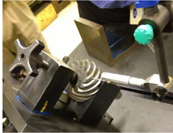
Figure 3.20 Measuring a pinion gear on Jenoptik probing system
