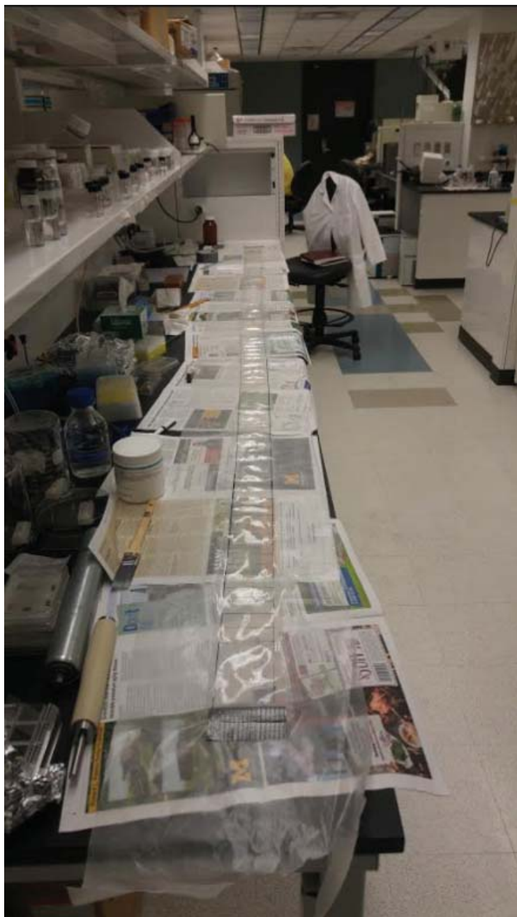
Figure 4-3. Photograph of the largest piece of film produced by Step 1. The film is 330 cm long, 10 cm wide, and \sim 150 \mu\text{m} thick. 515 mL of PVA solution was processed in the fabrication of this film. The leading 270 cm (415 mL solution) contains a colloid particle concentration of 3.0 mg/mL, the lagging 60 cm (100 mL solution) was processed with no particles in order to keep particles out of the nonuniformly stretched lagging endcap.
