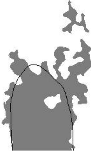
Figure 2.14: Example of an instantaneous flame surface for Case 3b (reactants in gray, products in white). The contour of average flame position is shown in black. This line indicates \bar{A}_F used in evaluating S_{T,GC,1} .
