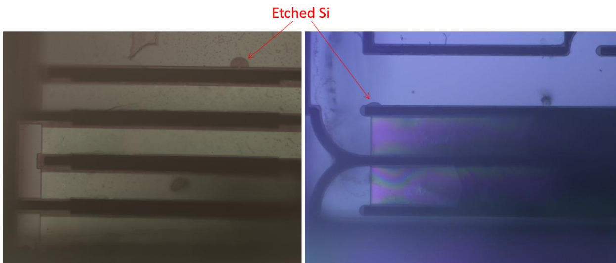
Figure 3.9. Etched silicon structure during XeF 2 etching due to voids in the SiO 2 -filled trenches
