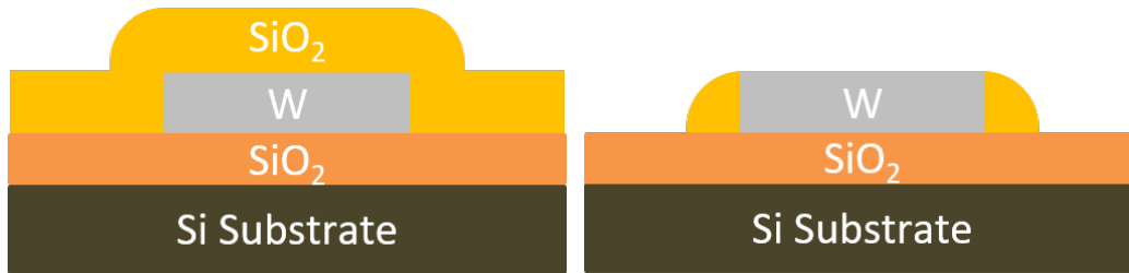
Figure 7-5: Schematic of spacer formation. Left: after isotropic deposition of SiO 2 . Right: after anisotropic etching of SiO 2 . The spacer is formed self-aligned along the sidewall of BE.
