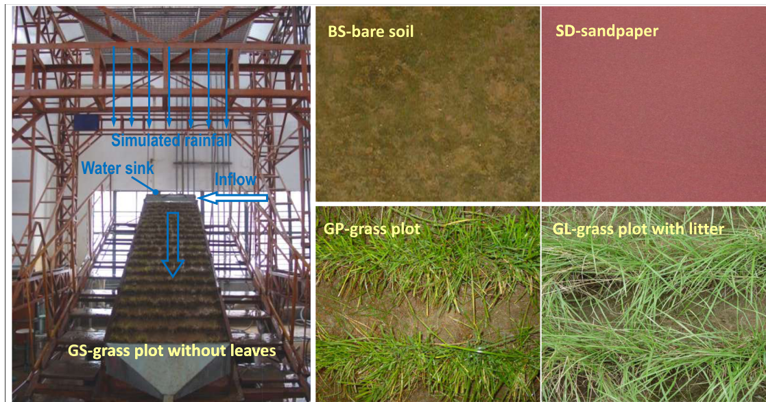
Figure 1. The scheme of this experimental setup and the tested plot surfaces.
