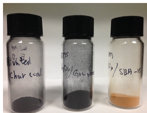
Figure 1. Pictorial representation of the \text{Fe}_3\text{O}_4 NPs on (from left to right) charcoal, single-layer graphene, and SBA-15.
