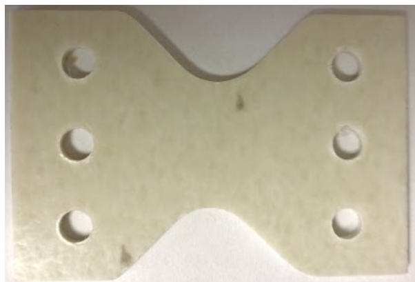
Figure 2.3: Butterfly shaped Arcan specimen
