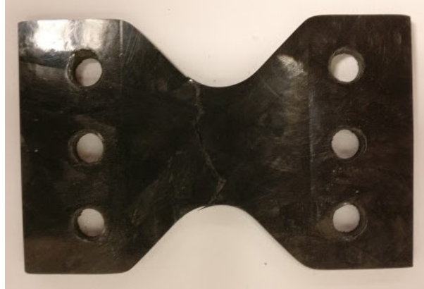
Figure 3.7: Damage in Carbon Fiber SMC-R under tensile load.
