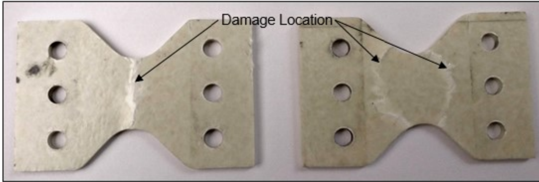
Figure 2.7: Damage locations in specimens at 0^\circ (left) and 45^\circ (right) loading angles
