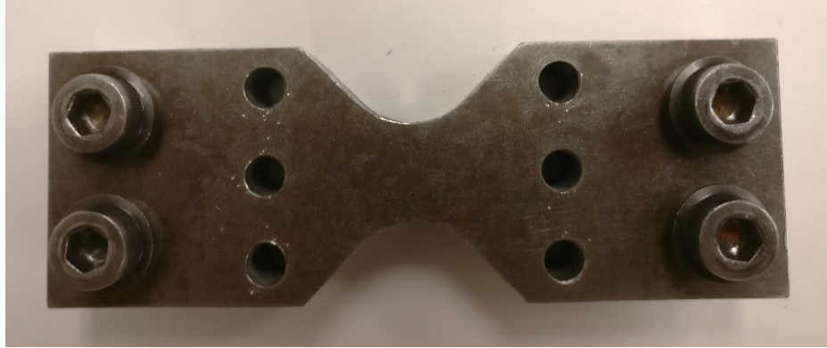
Figure 2.2: Template used to machine specimens.
