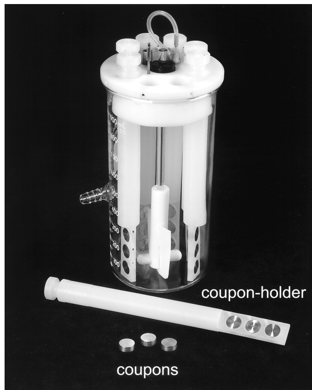
Fig. II.3. Open Flow Biofilm Model Systems. A. Modified Robbins Device (Azeredo et al. , 2017; Image © Claus Sternberg), and B. Centers for Disease Biofilm Reactor. Image acquired from Donlan et al. , 2004.
