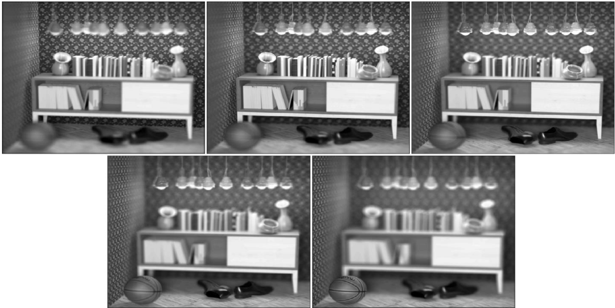
Figure 5.9 Focal stack images of the photorealistic scene. Sensor films are placed from the nearest to the farthest distances with respect to the camera lens, following the order from left to right, top to down.
