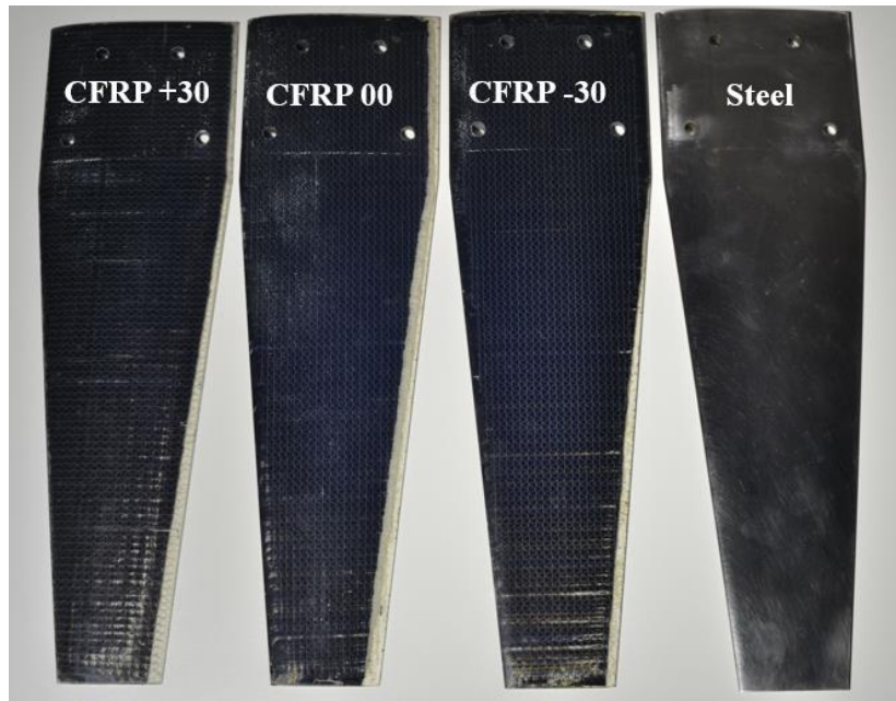
Figure 7.2: The three type II composite hydrofoils and the type II stainless steel hydrofoil used in experiments.
