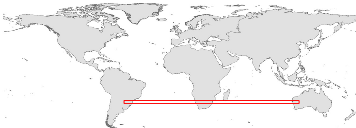
Figure 1.2 – Instantaneous homogeneity (full mixing): large grid cells, such as the red cell represented here (typical for latitudinal models), lead to a situation (artifact) in which emissions in e.g. Australia are immediately diluted and transferred to Africa and South America.
