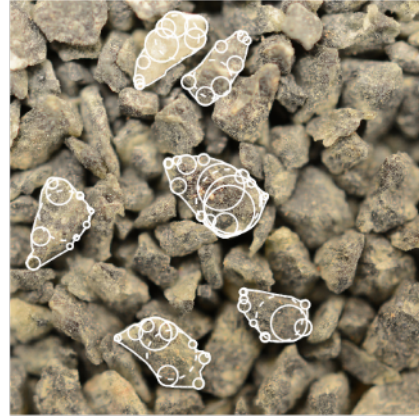
(b) Crushed Gabbro R = 0.23, \sigma = 0.08 S_{WL} = 0.56, \sigma = 0.14
