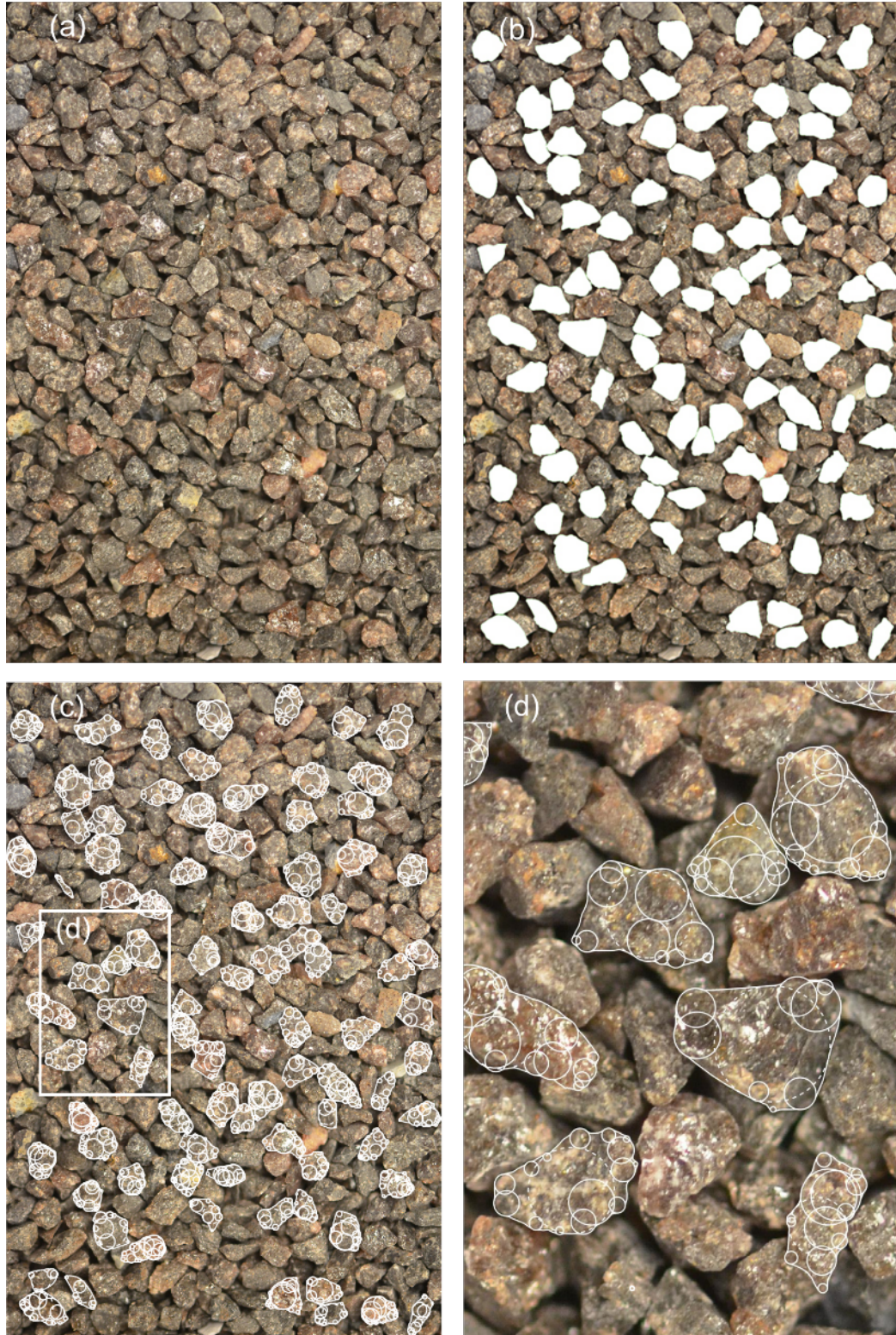
Figure 3.21 Circle fitting results for BFAO sand: (a) image of the three-dimensional assembly of BFAO; (b) delineated particles using Photoshop; (c and d) fitted corner circles (solid) and maximum inscribed circles (dashed).
