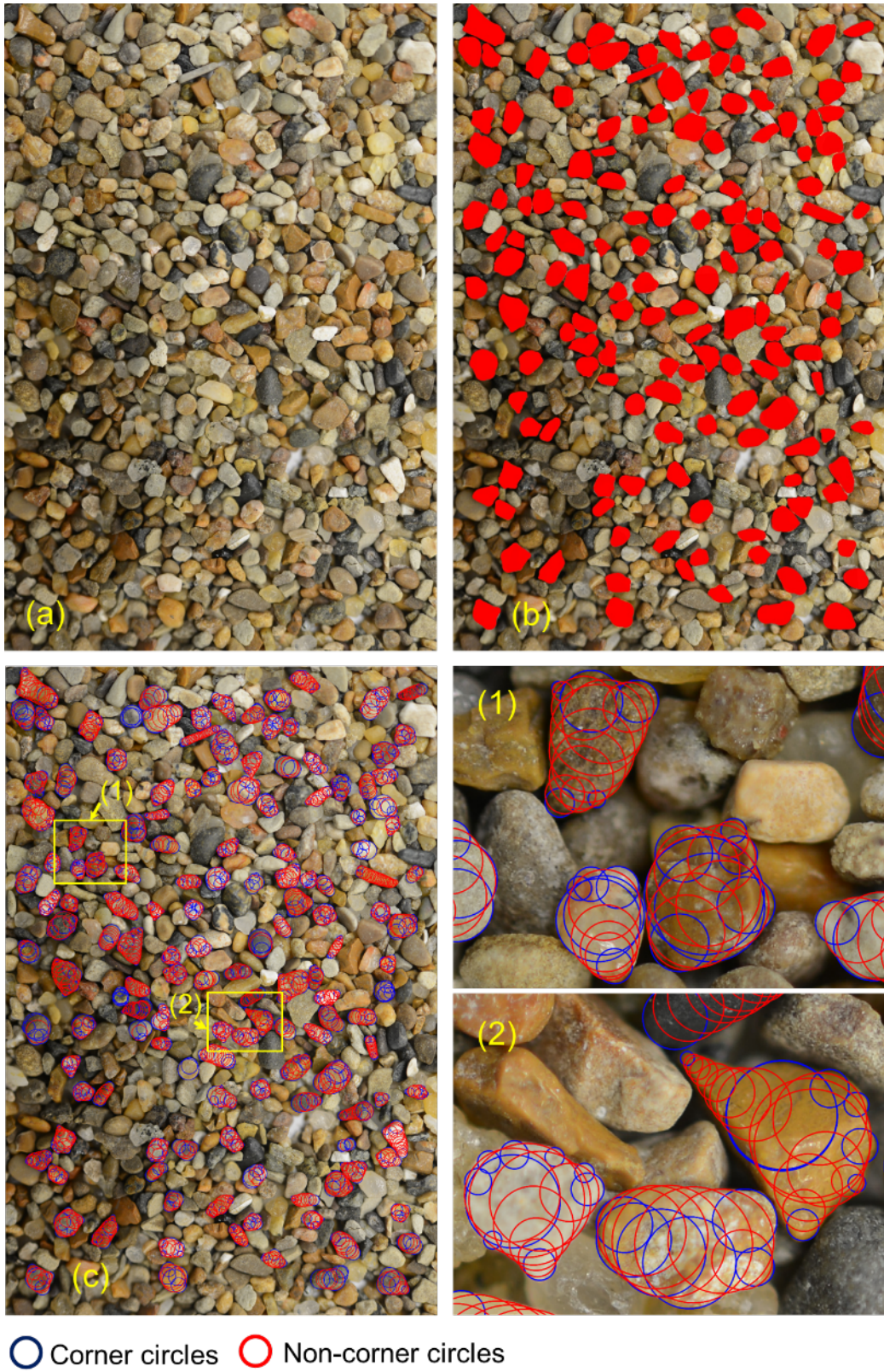
Figure 6.18 Clump generation from an image of a particle assembly.
