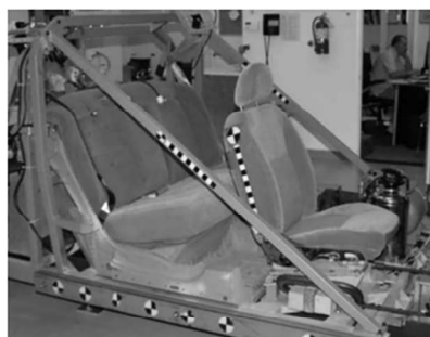
(a) Sled test buck
