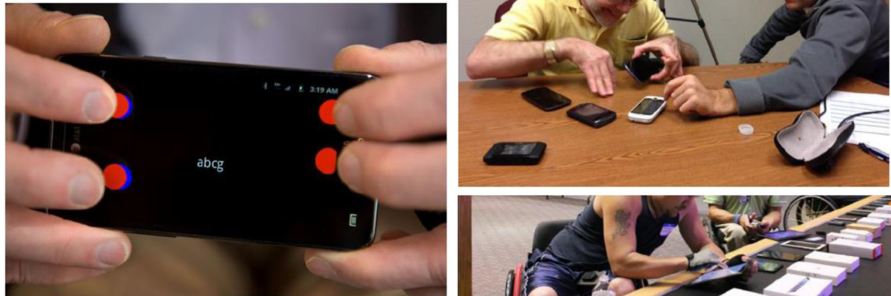
Fig. 12 Left: BrailleTouch smartphone app developed with support from the Wireless RERC's App Factory development project. The app allows the user to type braille directly on their iPhone or iPad, and send text messages, tweets, and emails from the touchscreen braille keyboard. You can also copy text that you enter using braille and paste it into any other app on your iPhone. Upper right: Helping consumer with cerebral palsy choose new smartphone. Lower right: Wireless RERC team conducting hands-on training session on built-in accessibility features in contemporary smartphones and tablets
