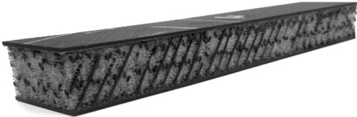
Figure 1. Sandwich composite made with a 3D fiber reinforced foam core. (Image not to scale.)
