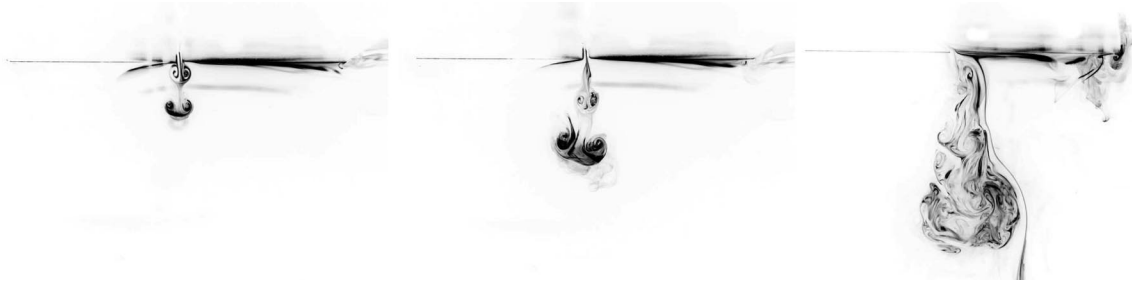
Fig. 7 Flow visualization for d = 0.05 , with 0.02c amplitude at 1 Hz oscillation. Gap dye injection (left) and one cycle later (middle) show vortex pairs producing a jet. Tip dye injection (right) shows vortex formation and flow entrainment towards the gap.
