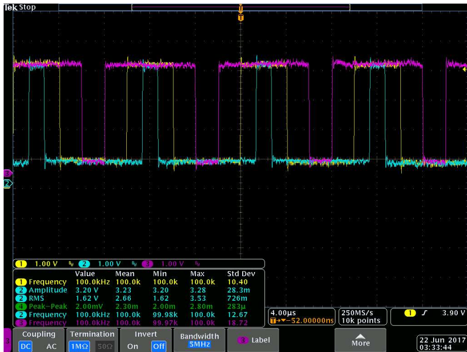
Figure 61. Three upper bridge PWM
