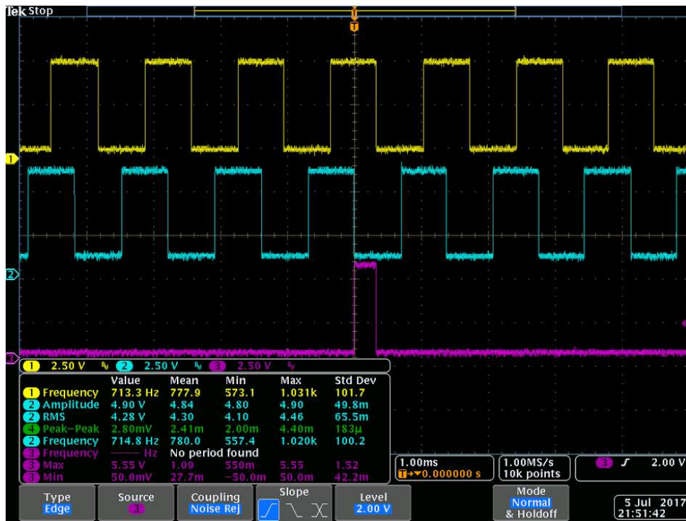
Figure 58. Phase A (yellow), Phase B (blue) and Index (red) signal
