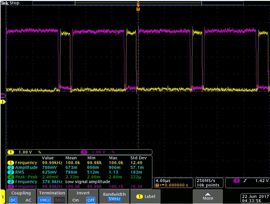
Figure 59. Complementary PWM signal
