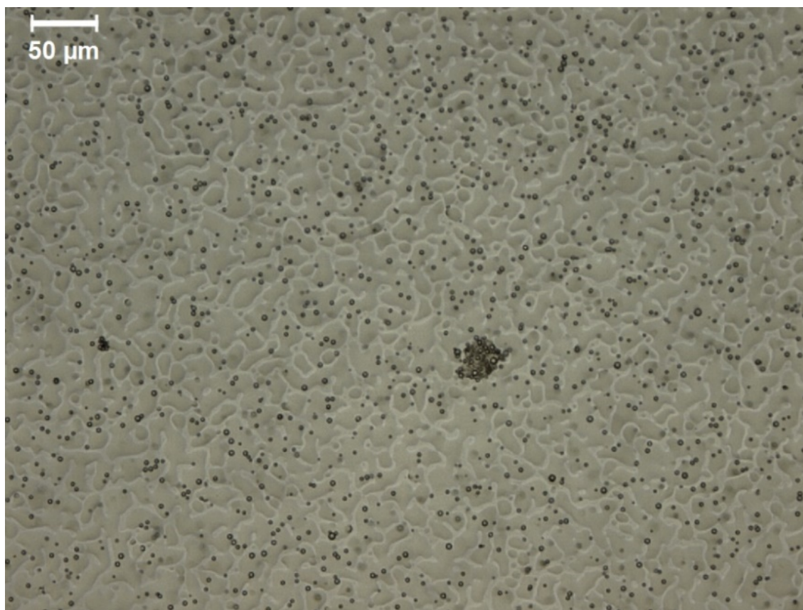
Figure 4.11. Islands and spherical domains of phase separated KTZ. The photo was taken at 40 min following the pH shift from 2 to 6.5.
