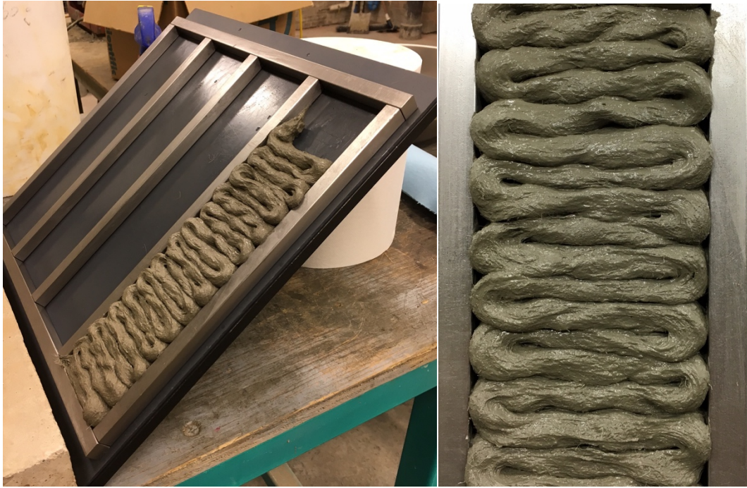
Figure 3.16: Preparation of the print pattern to be used in interlayer bonding testing of Mix 4 via the approximated 3D printing technique. Coupon shaped specimens were sectioned from the print pattern and tested in tension with the loading axis normal to the bond lines between filaments.
