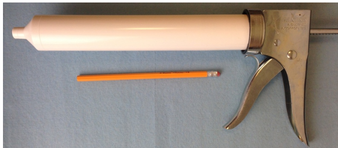
Figure 3.4: A mechanically actuated, manually operated caulk-gun apparatus, shown with a pencil for scale, was used as a means of extrusion for a small-scale approximation of the final step of the 3D printing process. Nozzle diameters 8-13mm were used.
