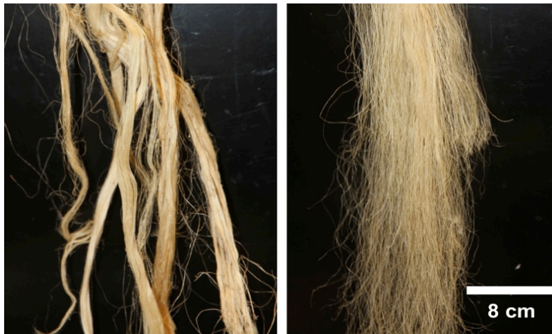
Figure 2.5: The appearance of the continuous curauá fibers prior to combing (left) and after combing (right), illustrating the effect of the treatment
