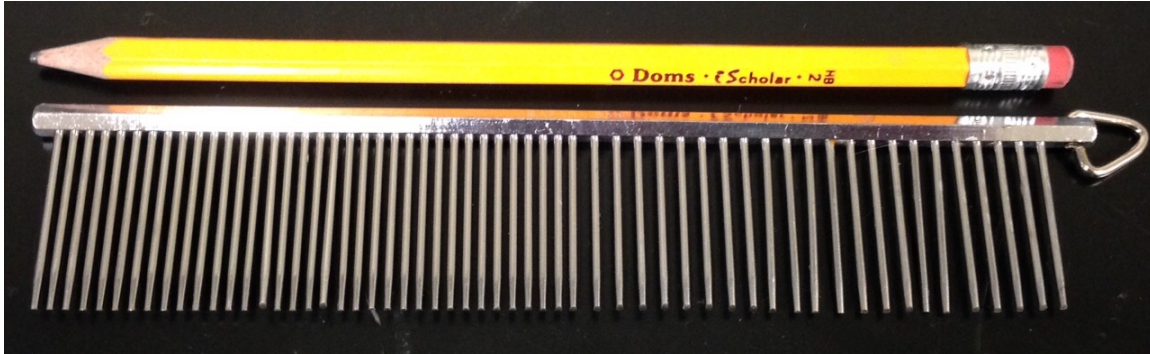
Figure 2.4: A straight-tooth, metallic comb used for a debundling treatment of continuous curauá fiber prior to chopping (shown with pencil for scale)
