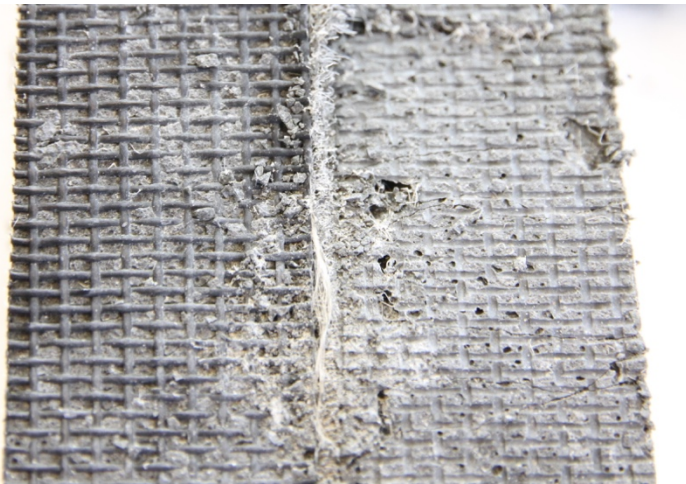
Figure 4.7: Opposing faces exposed after layer debonding and sectioning of a VCP-mesh specimen. Interlayer mineral bridges are formed through the mesh apertures and subsequently severed during loading, leaving a marked surface roughness that may contribute a desired resistance to layer sliding. Interfaces in the PP-mesh scheme have a similar appearance, but with larger mesh apertures and thus larger interlayer mineral bridges.
