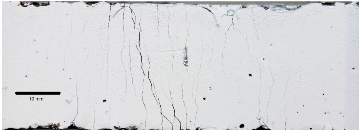
Figure 2.9: Distributed, multiple cracking pattern of the V0 curauá-ECC specimens under direct, uniaxial tensile loading (applied in lateral direction). The surface has been painted white prior to testing to enhance crack contrast.
