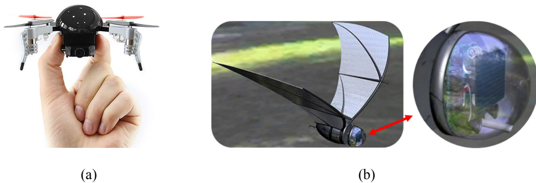
Figure 1.6. Diagram of micro-robotic platforms: (a) a micro quadcopter drone, and (b) a miniature mechanical bat for autonomous micro robotic applications. The navigation sensors for such miniature robotic platforms are required to have a low size, weight and power consumption (SWaP) with all-weather functionality.
