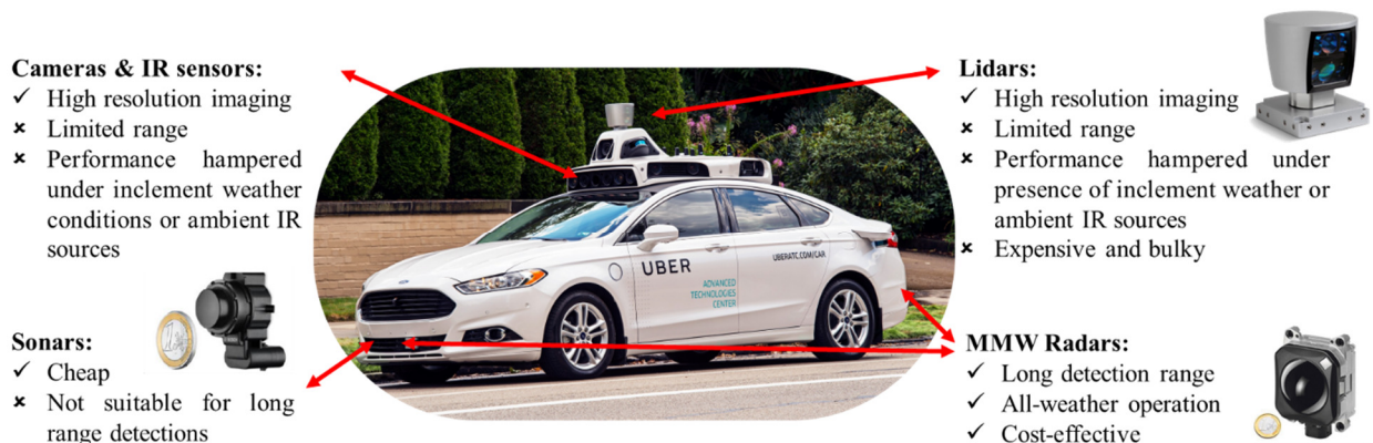
Figure 1.5. An overview of a state of the art self-driving car equipped with multiple different sensors for reliable navigation. The sensors are often too bulky, heavy, and power hungry, which makes them not suitable for ubiquitous autonomous applications.
