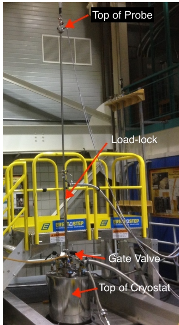
Figure 3.16: Photograph taken from the hybrid platform at the National High Magnetic Field Lab before the probe is loaded into the hybrid magnet. The sample stage at the bottom of the probe sits just above the gate valve. When the probe is loaded, the top of the probe will rest at the top of the load-lock chamber and the sample stage will be in the field center.
