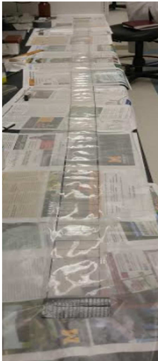
Figure 3. Photograph of a long PS embedded PVA film produced by Step 1. The film is 330 cm long, 10 cm wide, and \sim 150 \mu\text{m} thick. 515 mL of PVA solution was processed in the fabrication of this film. The leading 270 cm (415 mL solution) contains a colloid particle concentration of 3.0 mg/mL, the lagging 60 cm (100 mL solution) is free of particles.
