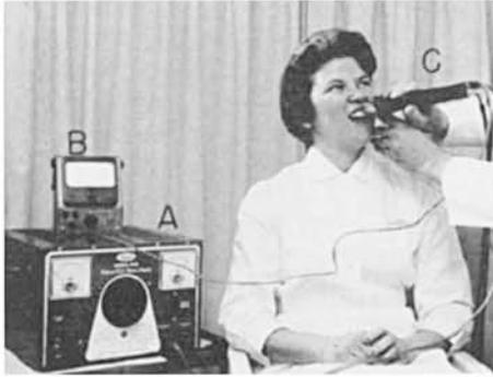
Fig. 5. Thermo-electric tooth stimulator system: (a) D. C. power supply. (b) Tele-thermometer. (c) Thermo-electric tooth stimulator.
