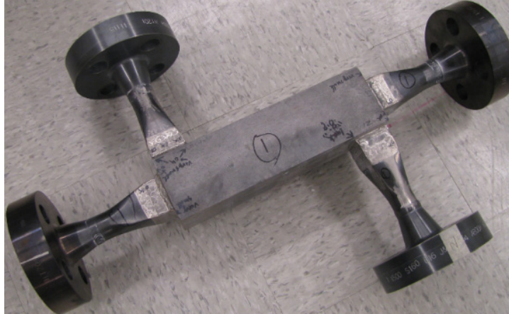
Figure 5-2. Straight-channel PCHE with four headers assembled (Mylavarapu, 2011).
