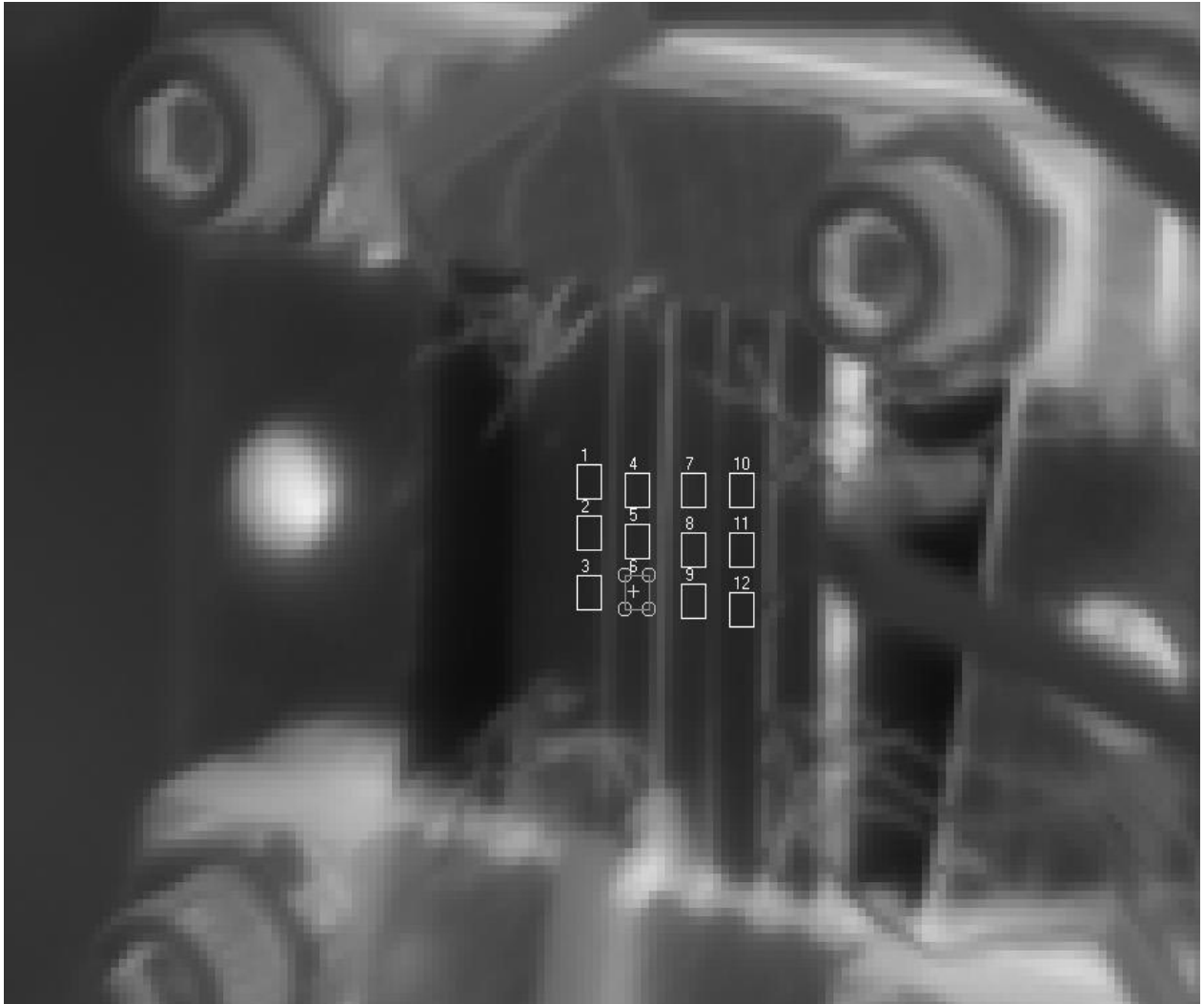
Figure 4.15 An image taken from the FLIR 2D imager of a heated irradiation stage with three square AOIs on each sample.
