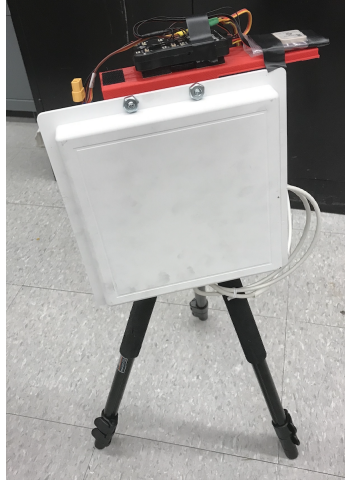
Figure 5.22: Antenna tracker with patch antenna
