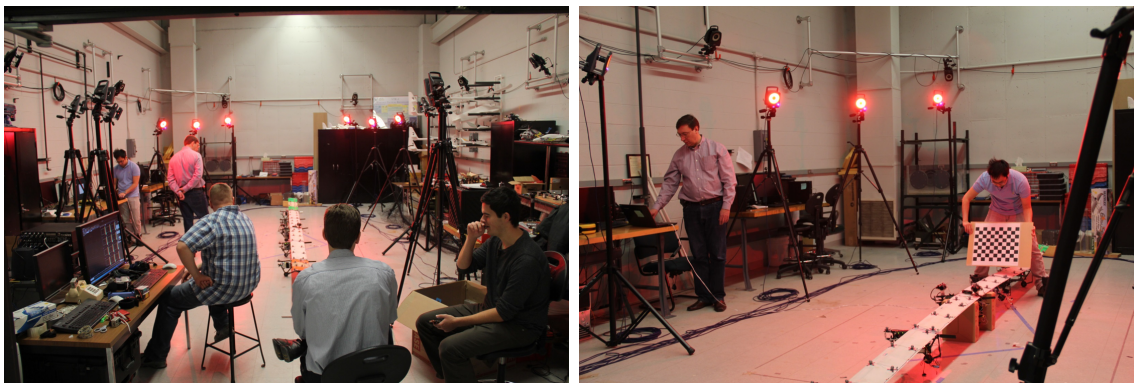
Figure 3.13: Vicon T-40 cameras mounted on tripods around the testing area
