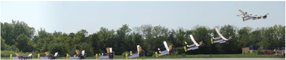
Figure 5.1: X-HALE aeroelastic testbed vehicle takeoff sequence [1]
