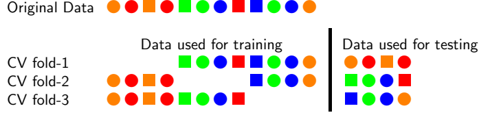
Figure 2.7: Schematic describing the process of cross-validation (CV). The example uses a 3-fold CV. The figure is adapted from https://tex.stackexchange.com/a/154121 .
