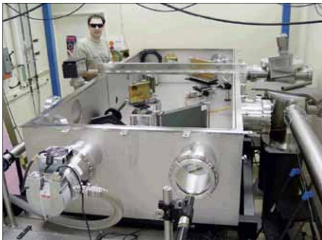
The Hercules laser compression chamber
