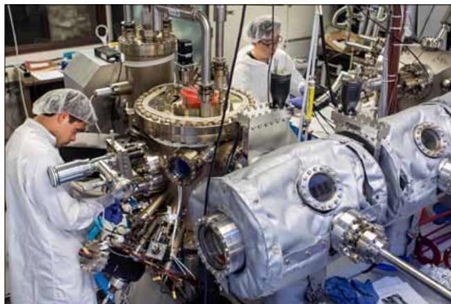
Fast neutron generator
