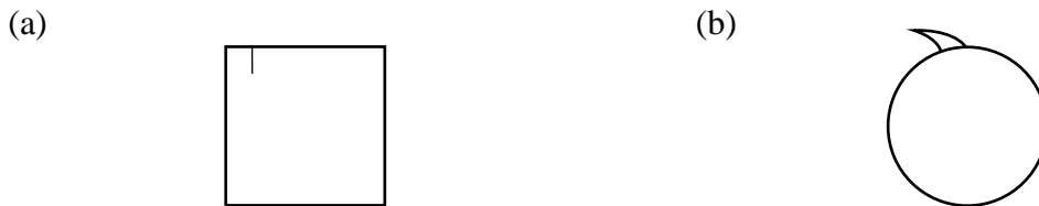
Figure A.0.2 (a) Schematics of marking cut to indicate the orientation of the film for in-situ cell fabrication. In this case, when put in this orientation, the front surface is the “+” side of the film and the back surface is the “-” side of the film, so that there would be a polarization voltage when the film is squeezed with pressure. (b) Schematics of marking tail to indication the orientation of the film for coin cell fabrication. In this case, when put in this orientation, the front surface is the “+” side of the film and the back surface is the “-” side of the film, so that there would be a polarization voltage when the film is squeezed with pressure.
