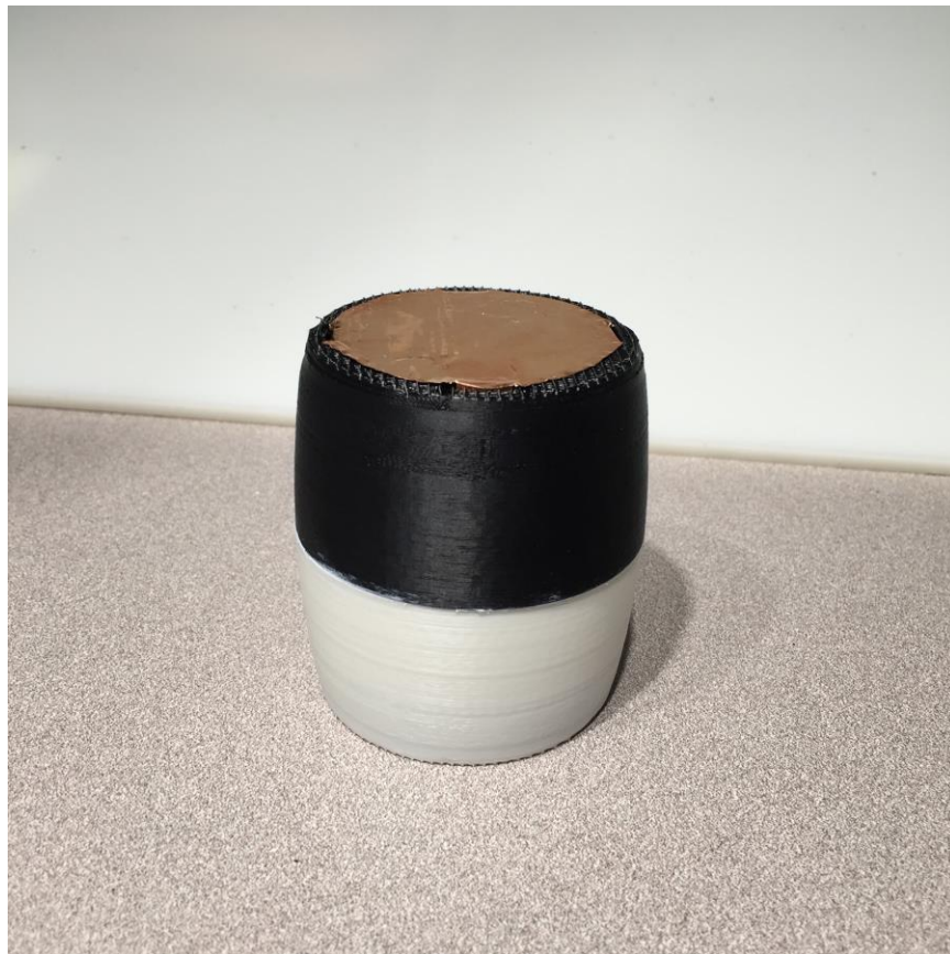
Figure 6.10 A sample cylindrical bubble battery
