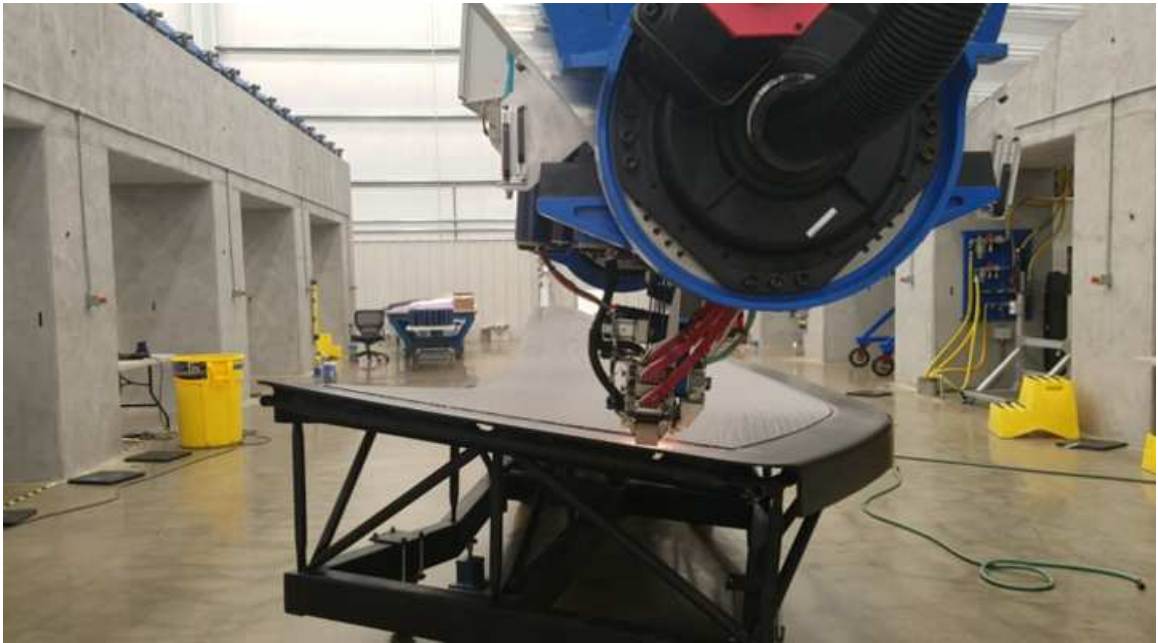
(a) Wingbox skins being laid up by AFP machine
