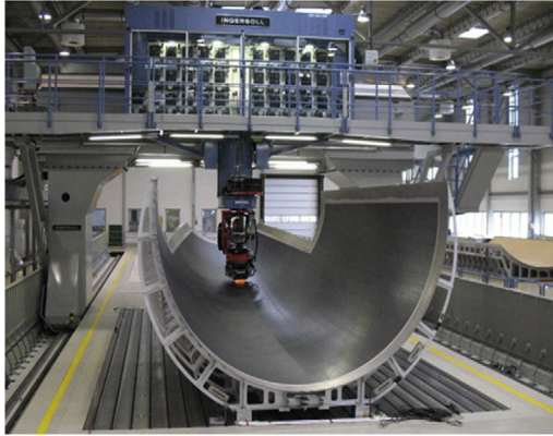
(a) AFP layup of fuselage section [10]
