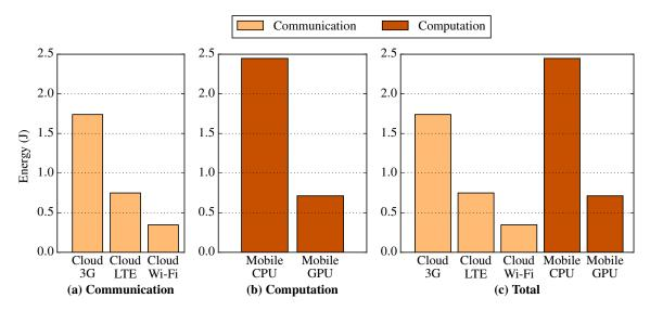
Figure 3.2: Mobile energy breakdown for AlexNet (image classification). Mobile device consumes more energy transferring data via LTE and 3G than computing locally on the GPU.
