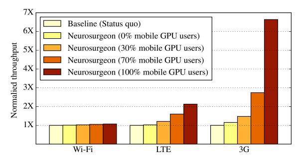
Figure 3.14: Datacenter throughput improvement achieved by Neurosurgeon over the status quo approach. Higher throughput improvement is achieved by Neurosurgeon for cellular networks (LTE and 3G) and as more mobile devices are equipped with GPUs.
