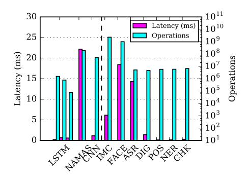
Figure 4.3: Latency and FLOPS of NLP and traditional NNs on GPU
