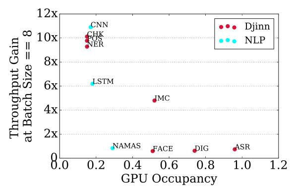
Figure 4.5: Occupancy and throughput gain of applying DjiNN's batching technique
