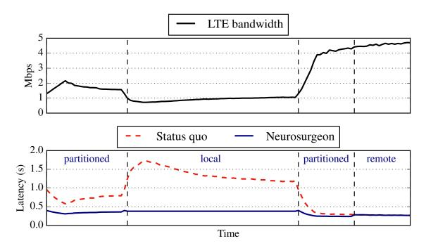
Figure 3.12: The top graph shows bandwidth variance using a LTE network. The bottom graph shows the latency of AlexNet (IMC) of the status quo and Neurosurgeon. Neurosurgeon's decisions are annotated on the bottom graph. Neurosurgeon provides consistent latency by adjusting its partitioned execution based on the available bandwidth.
