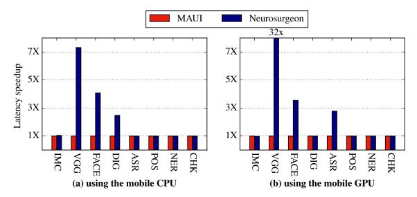
Figure 3.11: Latency speedup achieved by Neurosurgeon vs. MAUI [35]. For MAUI, we assume the optimal programmer annotation that achieves minimal program state transfer. Neurosurgeon outperforms MAUI by up to  $32 \times$  and  $1.9 \times$  on average.
