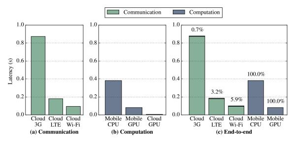
Figure 3.1: Latency breakdown for AlexNet (image classification). The cloud-only approach is often slower than mobile execution due to the high data transfer overhead.
