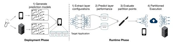
Figure 3.8: Overview of Neurosurgeon. At deployment, Neurosurgeon generates prediction models for each layer type. During runtime, Neurosurgeon predicts each layer's latency/energy cost based on the layer's type and configuration, and selects the best partition point based on various dynamic factors.
