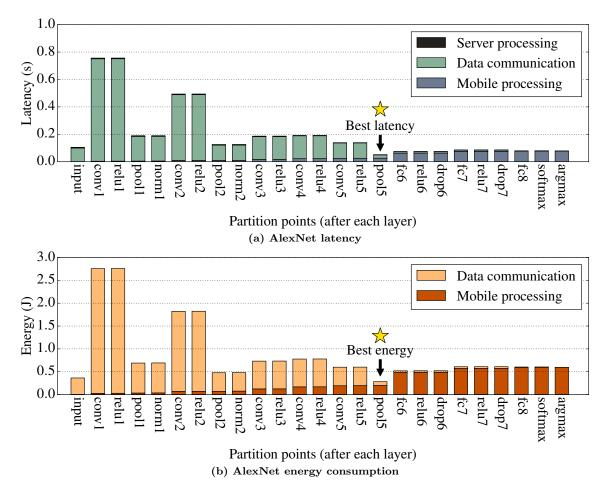
Figure 3.4: End-to-end latency and mobile energy consumption when choosing different partition points. After the execution of every layer is considered a partition point. Each bar represents the total latency (a) or mobile energy (b) if the DNN is partitioned after the layer marked on the X-axis. The left-most bar represents cloud-only processing and the right-most bar represents mobile-only processing. The partition points for best latency and mobile energy are annotated.
