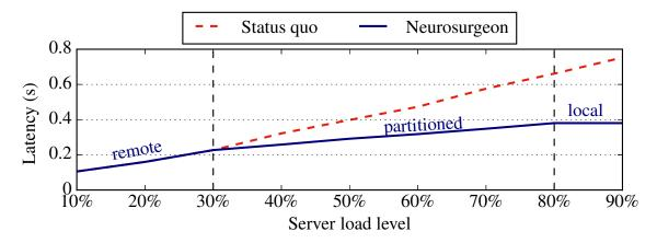
Figure 3.13: Neurosurgeon adjusts its partitioned execution as the result of varying datacenter load.
