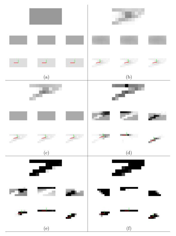
Figure 3.6: Optimization iterative details for the cantilever example at (a) iteration 1; (b) iteration 5; (c) iteration 10; (d) iteration 15; (e) iteration 30; and (f) iteration 74.
