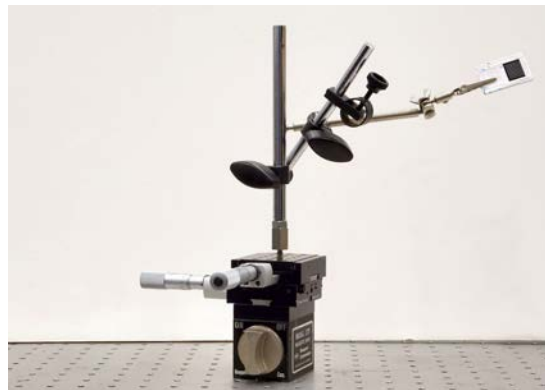
Figure 1.17: An expedient way to hold a calibration grid for 3-D DIC calibration is the magnetic base stand commonly used for dial gauges. Note that the calibration grid is shrouded in tape on the perimeter to cushion a fall in the event of dropping the grid.
