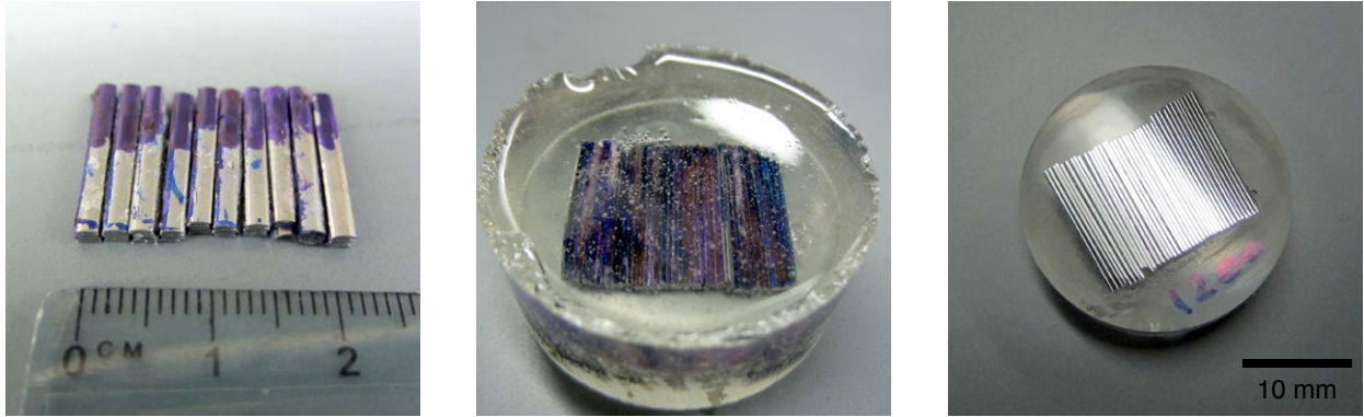
(a) The forty quarter sections of tube (in ten stacks of four) before mounting.
