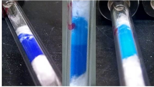
Figure 2.3. Packed columns of HKUST-1 and the observed color change of the material from before (left), during (middle), and after (right) sorption of DME via flowing a 2% DME in MeCl mixture.
