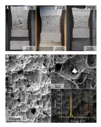
**Figure 8:** The impact of adding a single element is shown by the highly differentiated fracture surface. Electron images of (a) NiFeCrCo and (b) NiFeCrCoMn are shown at their fracture surfaces. Image courtesy of Dr. Carl Koch (North Carolina State University).<sup>69</sup>
