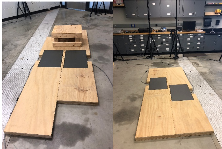
Figure 16: Force plate position on walkway for (a) Jump trial (b) Run trial
