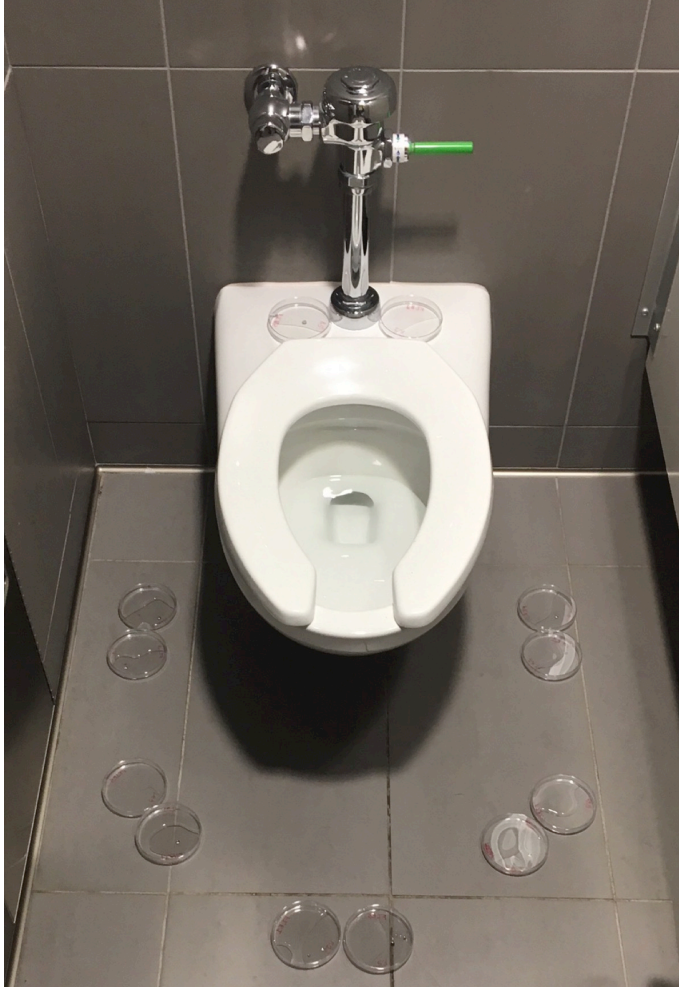
Figure C-2. Conventional flush toilet with petri dish layout to collect virus-laden droplets. Two dishes for each location (starting at the back of the toilet and rotating clockwise, back, right, front right, front, front left, left) are used to collect samples 1 minute and 5 minutes after flushing. Experiments were completed in triplicate.
