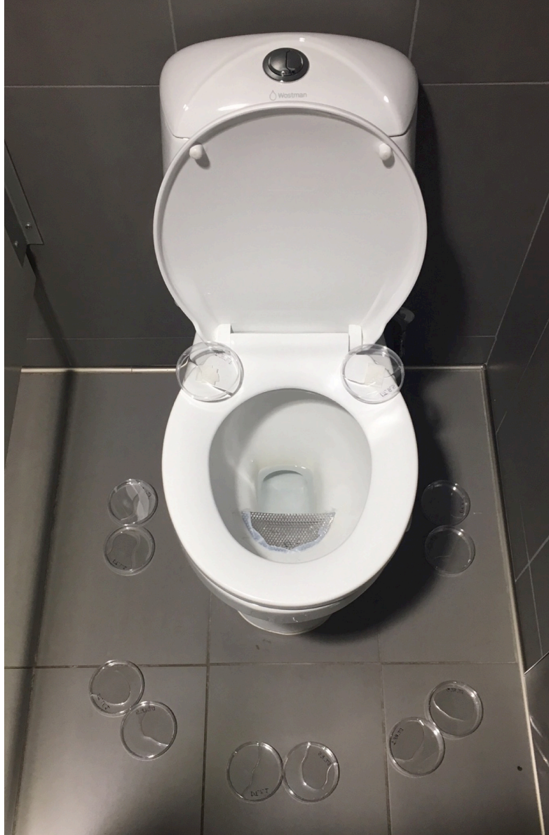
Figure C-1. Urine-diverting toilet with petri dish layout to collect virus-laden droplets. Two dishes for each location (starting at the back of the toilet and rotating clockwise: back, right, front right, front, front left, left) are used to collect samples 1 minute and 5 minutes after flushing. Experiments were completed in triplicate. Urine diverting toilets differ from conventional toilets with a separate front bowl and plumbing to collect urine. The mesh screen shown here was added to the toilet to prevent other items besides urine from entering the bowl and provide easier cleaning for when this occurs.
