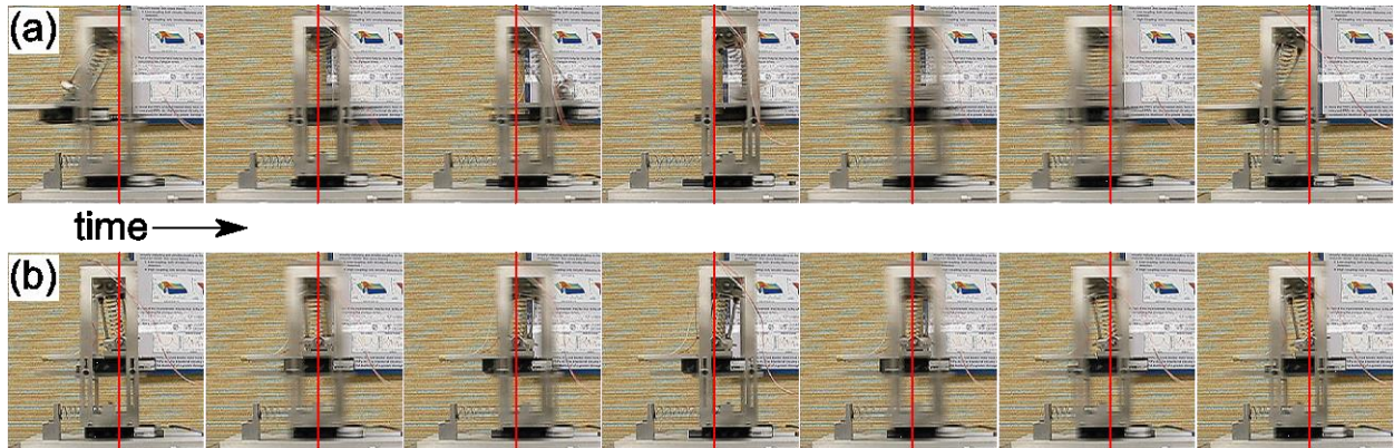
Figure 27. Frame by frame photographs of one excitation period for coupled system having f_2 : a) in-phase response at 3 Hz; b) out-of-phase response at 5 Hz. Vertical red lines are identically positioned throughout the timeseries to serve as position references.
