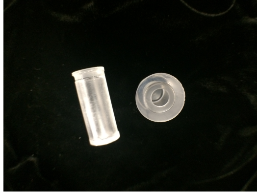
Figure 5.18: Third stilbene prototype manufactured with a cylindrical body and two endcaps to increase the structural stability of the cell.
