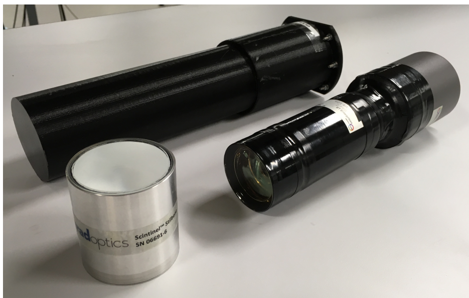
Figure 2.5: (Bottom left) InRad optics stilbene encased in aluminum, (bottom right) ET Enterprises 9214b PMT, and (top) 3D printed case for detector assembly. The PMT and stilbene scintillator are coupled with optical grease and secured with black electrical tape to make the system light tight.
