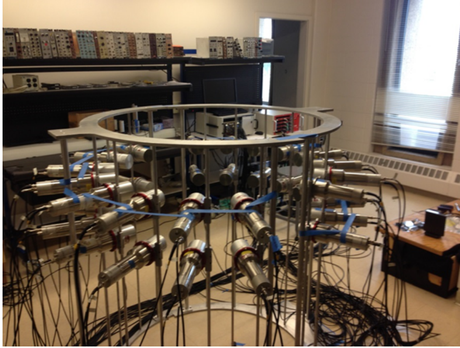
Figure 5.1: A photograph of the detector holder and 32 detectors, 14 - 7.62\varnothing \times 7.62 cm EJ-309's, 8 - 7.62\varnothing \times 5.08 cm EJ-309's, and 8 - 7.62\varnothing \times 7.62 cm NaI(Tl) scintillators.
